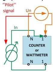
Used with a voltage source, the POC-1200 allows to control and calibrate electric meter and wattmeter.
